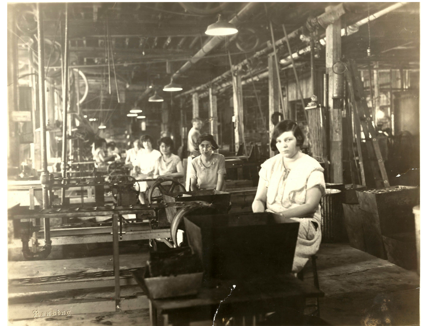
Ring Press Department Ring Press Department at Continental Diamond Fibre Factory, by A. H. Reading, c. 1931-1935. This photograph shows women working in the ring press department of the Continental Diamond Fibre factory in Valparaiso. While the factory didn't actually make diamonds, it did manufacture mica, vulcanized fiber, and bakelite for use in electrical insulation.
